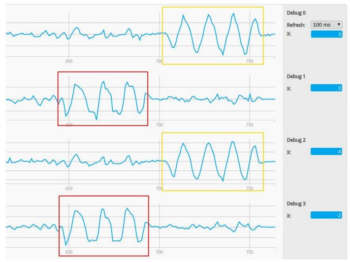
Change the "align\_opflow" parameter in CLI and retry the procedure until your Debug 0 looks similar to Debug 2 and Debug 1 is similar to Debug 3.
